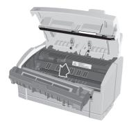
Do not expose the image drum to strong light. Do not touch the image drum's green surface.
